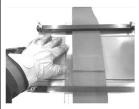
Make sure the joints are not bent at scale, to be fixed in the belt clamp the belt.
