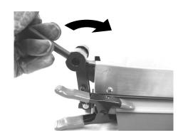
• The cam is hitch to the frame. And the clamp lever is turn to the main body side.
