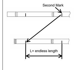
When consecutively making endless belts, obtain required belt length and from the second mark made at the preceding finger joint, measure out the required belt length and make another mark. Repeat the above process. By doing this, punching can always be made at the right position and there will be no wasted belt.
